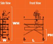
Base Dimensions (L x W) Max Platform Height (PH) Max Working Height (WH) Max Working Load Weight (kg)
