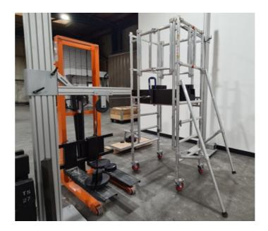
The tests carried out are strenuous and specific to this kind of equipment, in particular platform strength, side-loading and anti-skid ensure an item will be safe for use within any environment - whether it's painting a ceiling, servicing a duct or drilling into a structure, the podium is designed and tested to ensure the operator has the safest and most suitable product available to them.
